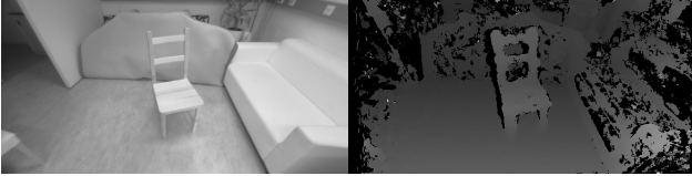
Fig. 4. Left rectified input image and corresponding disparity map.
